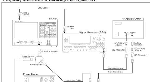
Figure 2-4 Frequency Measurement Test setup 1 for Option 011
