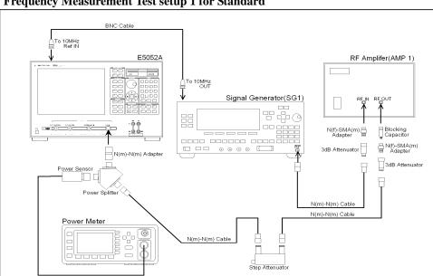
Figure 2-2 Frequency Measurement Test setup 1 for Standard
